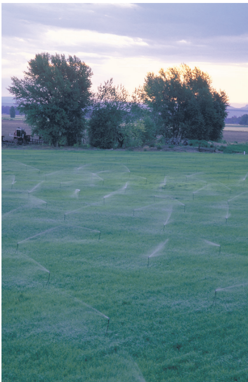
For irrigation of field crops. The R10T Rotator® is used as part of a portable irrigation system that utilizes polyethylene pipe for laterals in combination with the Nelson FT5 feedtube assembly.
